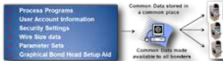
Bonder Data such as user accounts, security settings, bond parameter sets and wire size data can be transferred from a host to all machines to ensure commonality and production line control
